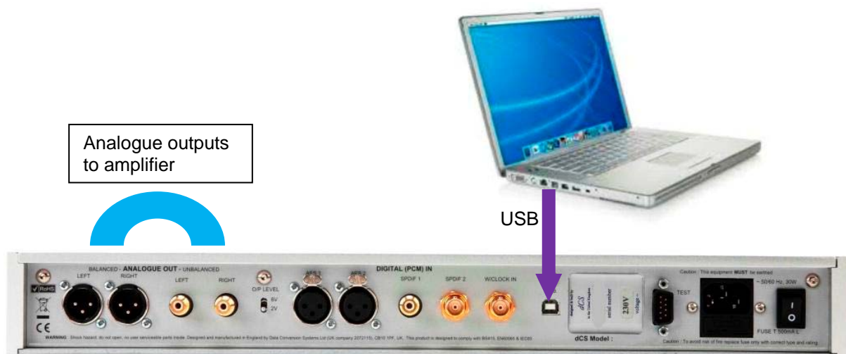
Figure 1 – Connecting the USB interface.
