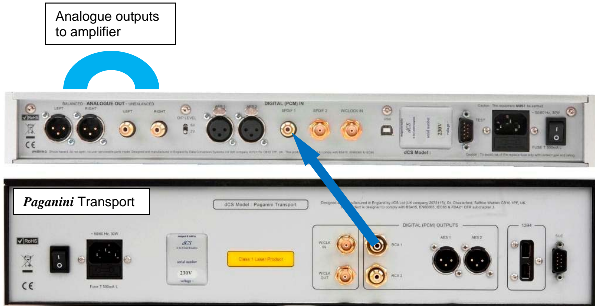
Figure 2 – Connecting an SPDIF interface.
